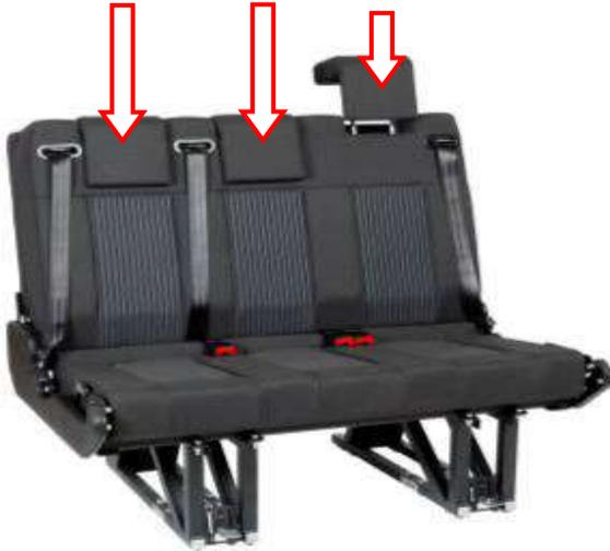
2. Pull the front part of the seat section upwards, the head restraints must be retracted
