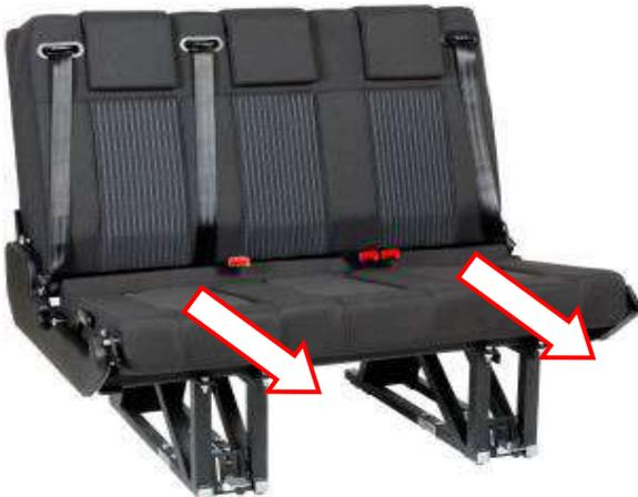
4. Fold the seat section upwards
