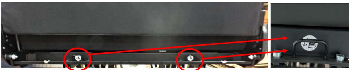
The Top-Tether attachment eyelets are located on the back of the bench, below the back cushion on the rear leg attachment.
